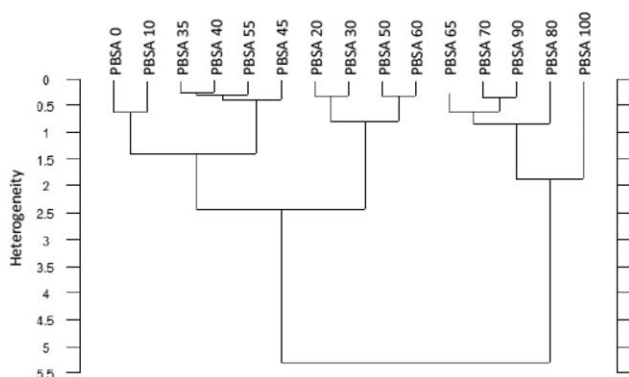
Figure 4. Hierarchical clustering of the 15 PBSA/PEO films based on ATR-FTIR spectra analysis (full spectral range 400–4000 \text{cm}^{-1} ).
